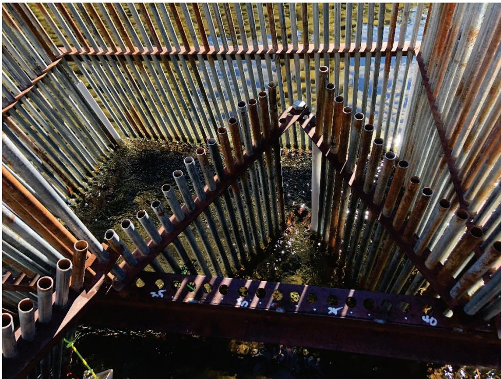
**Figure 6. Upstream trap box. A similar configuration was used for the first stage of the downstream trap. Photo credit: Mark Nelson.**
